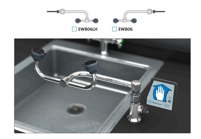
**Application:** Eyewash for mounting on counter next to sink. Spray heads swivel 90 degrees from storage to operational position. Water flow is activated by flag handle.
