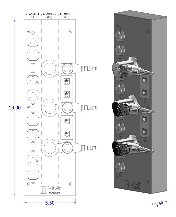
Example type 2C configured as shown, p/n SH-2CWS043C
